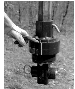
Top and bottom each has six holes tapped 1/2" - 13 on a 5 1/4" bolt circle.
